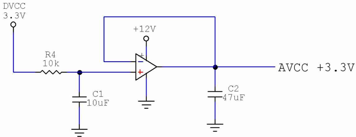
**Figure 4: AVCC +3.3V Filter and Regulator**
